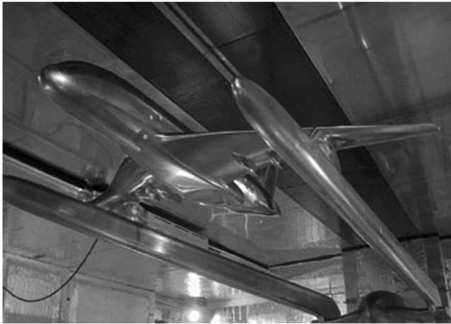
Fig. 1 Photograph of a wind-tunnel test model suspended with twin stings.
